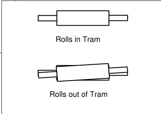
uneven as well. The same is true for rolls operated out of tram. Normally the tram adjustment will be set only when rolls are changed, or in the event of some significant upset condition (such as lost elevator buckets and bolts appearing in the nip of the rolls).
