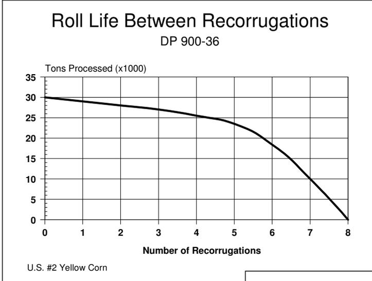
Larger diameter rolls will process more tons before recorruagation, and will have a deeper roll chill or hard working surface. Because of the better nip angle, large diameter rolls are often used in flaking operations where roll corruagations may be very fine to prevent cutting the grain while making thin, uniform flakes. Larger diameter rolls must also be used in machines with longer rolls to maintain the degree of stiffness required for holding the rolls in position.
