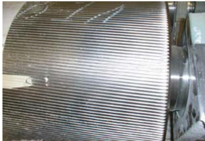
when roll adjustments are made, running the rolls together with pressure and no feed will greatly accelerate roll wear. Evidence of roll to roll contact would be corrugations with tops that appear flat, with sharp or broken edges. There will normally be some circumferential grooving or scratches in the rolls as well. Roll to roll contact is most obvious due to the noise
