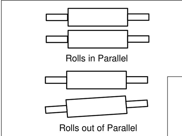
In order to achieve best roll life and consistent performance from end to end the rolls must be parallel and tram. If rolls are allowed to operate out of parallel, not only is the product inconsistent (fine on one end, coarse on the other) but the roll wear will be
